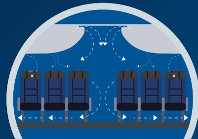
Modeling shows the airflow pattern, exchange rate, HEPA filtration, and forward-facing seats create conditions equivalent to 7 to 15 feet of social distancing, even for adjacent seats.
